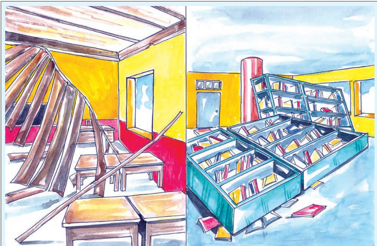
Sketch showing collapse of false ceiling in a school. Poor performance of NSE's in earthquake is avoidable through design.
